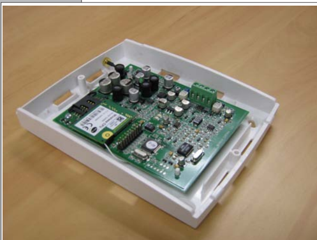
GSM Terminal Internal View
